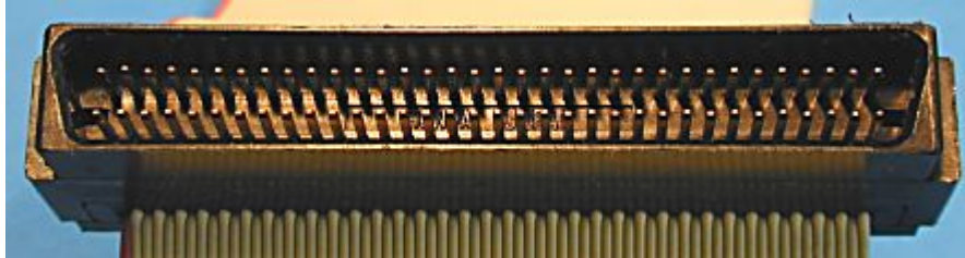
Figure 13 - A male, internal, high-density 68-pin connector
