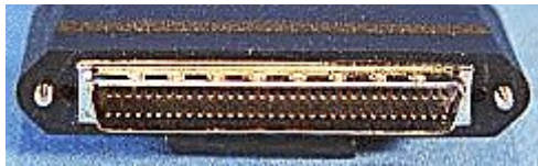
Figure 10 - Male 50-pin (above) and 68-pin external high density connectors
