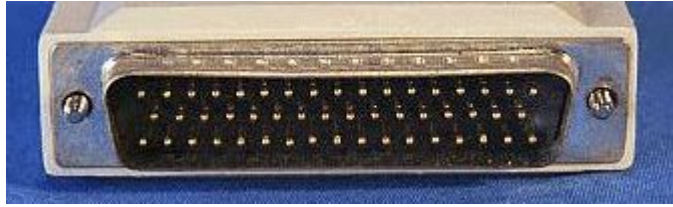
Figure 8 - A male DD-50 SCSI connector
