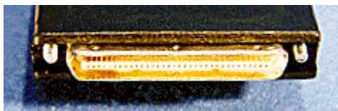
Figure 11 - A male 68-pin VHDCI connector
